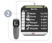
Within seconds, the exact result is displayed on the back side of the device.
