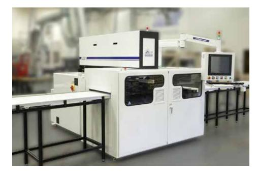
handling technology for precision cut-to-print registration and transfer of complete piece parts. The system can be integrated with commercial and packaging printers to create a complete digital workflow from start to finish. A variety of options are available to enhance functionality and optimize your initial equipment investment.
