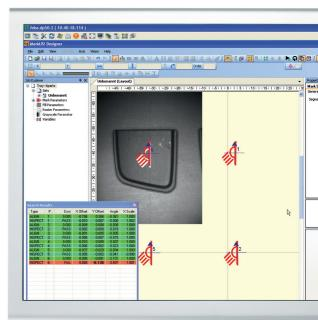
Verification report: The last part failed inspection as the Y position exceeded the 0.1 mm tolerance.
