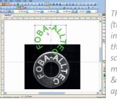
The P&S camera focuses (through the lens) on the marking field\*, creates an image of the part, and displays it on the screen. The user creates the marking and places it (via drag & drop) where it should be
