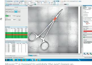
Mosaic<sup>™</sup> is trained to validate the part (green results) and align a laser mark on a pair of forceps. Although the part is randomly placed under the laser, the system is capable of aligning the mark to the part.
