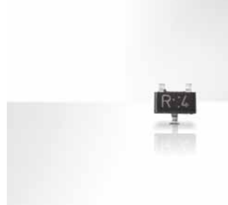
Microchip (IC) components On top: epoxy resin, 6x6 mm marking field, marking time 45 ms Below: epoxy resin, 2x1 mm marking field, marking time 10 ms
