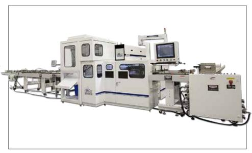
CIM systems use patented laser control software and advanced vision technology to assure precise, repeatable cut-to-print registration. Instant job change at production speed is accomplished through programming or reading printed bar codes. The integrated robotic material handling system removes scrap and feeds trimmed printed material to the proprietary folding and gluing system specially designed by Kluge to accommodate job changeovers.
