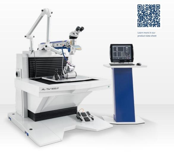
The AL-TW laser system has the laser source (Nd:YAG or fiber laser) integrated in the table. The workpieces can be precisely controlled in 3 axes (X, Y, Z) during welding. In addition, a rotary axis for circumferential welding is available as an option.
