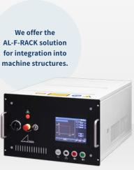
The FIBER LASER AL-F is available with 300, 450, 600, 900 W. We recommend fiber lasers for sheet metal processing, for deep penetration welding, for CW welding and for reproducible welding results thanks to the integrated power monitoring. The fiber source is characterized by high energy efficiency.
