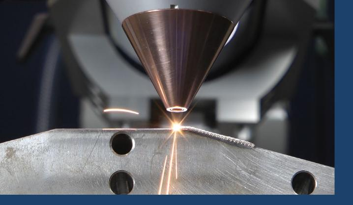
For powder deposition welding you need the powder nozzle LASERHEAD P and the powder feeder AL-PF.
