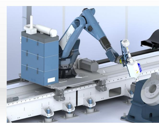
powder deposition welding. Only one controller is required to control all axes. As a result, the operation of the hardening system also with the addition of powder deposition welding - can be learned very easily and
