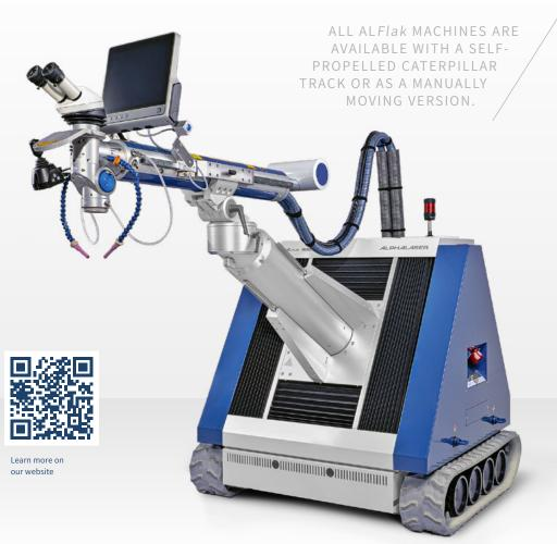
The **AL***Flak* is also available with fiber laser sources: 300, 450, 600, 900 and even 1200 W. The fiber source model is recommended if your application requires a validated process, if you wish to weld using CW (continuous wave) method or pulses. For deep welding in sheet metal fabrication, for laser cladding. And also, for melting thick wire diameters up to 2.0 mm in the high performance classes.
