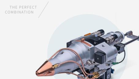
The powder passage is dependent on the power of the laser system: the stronger the laser, the more powder can be melted. The powder delivery rate is precisely controlled via the platen speed. The application rate for e.g. steel is approx. 500 - 600 g per hour.
