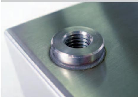
Circular welding at stainless steel housing
