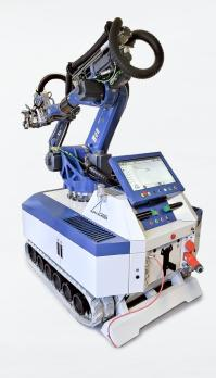
The laser beam precisely follows the workpiece contour in free 3D movements. This makes it easy to harden closing edges, grain structures, dimples or individual points.
