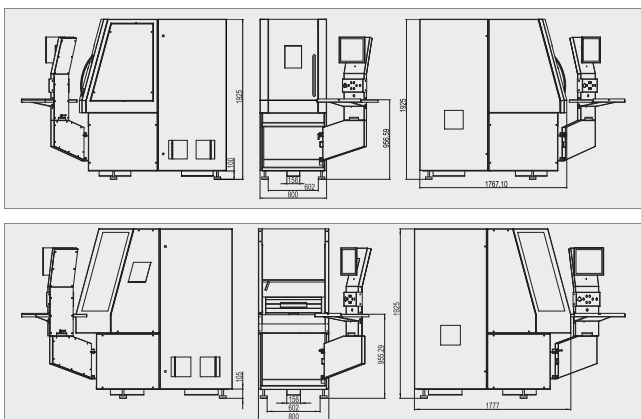
Top left: G3 with X/Y cross table and sliding door Bottom left: G3 with rotary table (dimensions in mm)
